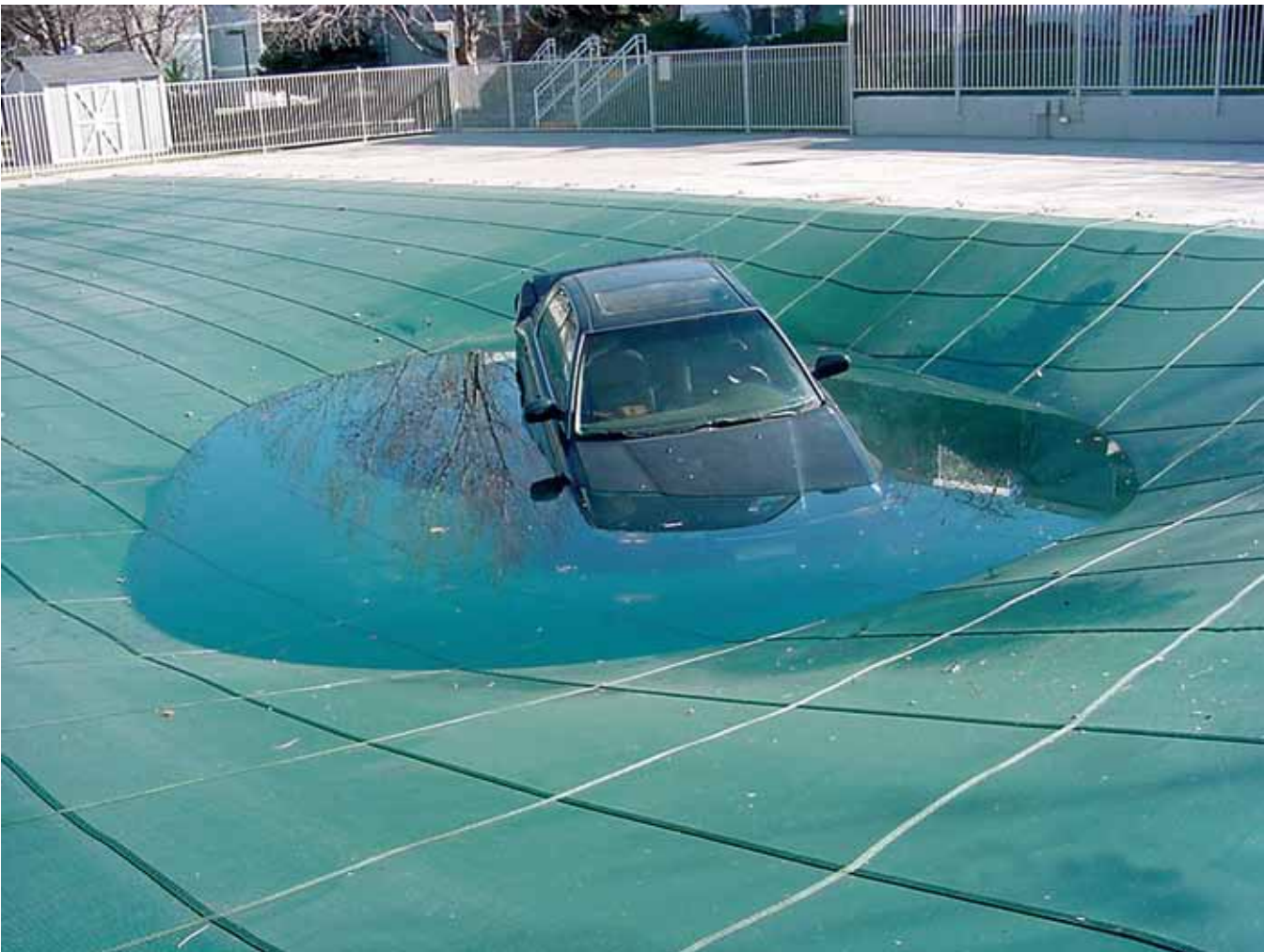
3212 pound vehicle accidentally driven onto a 40' x 80' Dura-Mesh safety cover. Can you spot where the driver walked off to safety?
